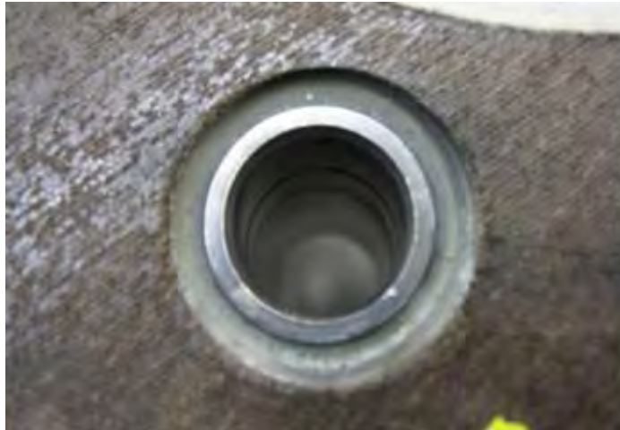
Figure 1: Example Installed Non-Conforming Sleeve Bushing PN 406-010-105-101
