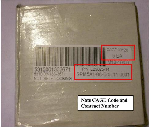
Figure 3: Example of Non-Conforming Main Rotor Latch Nut packaging
