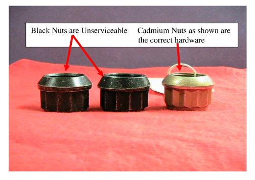
Figure 2: Comparison Non-Conforming MR Nuts with Conforming Nut
