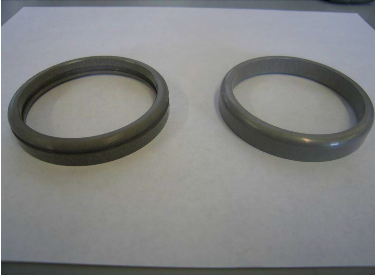
Example of Obsolete Ring (Left), and Serviceable Ring (Right)
