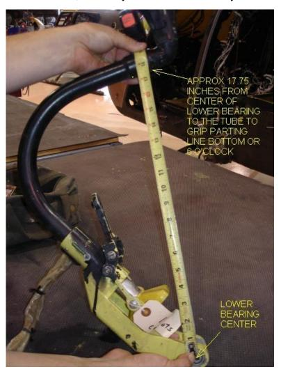
The photo below is an example of a non-conforming Co-pilot Cyclic Control Tube: Note length as measured.
